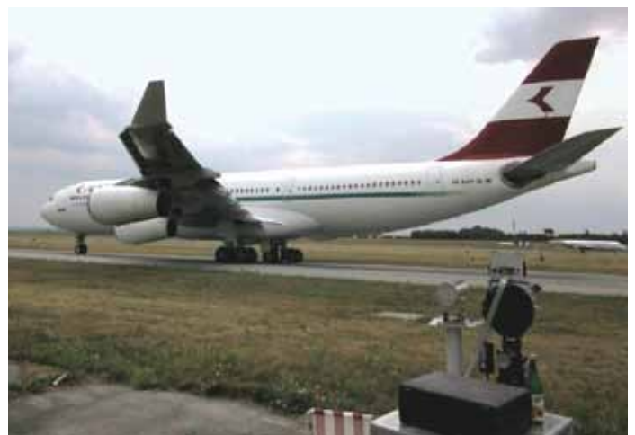
Figure 4: Aircraft plume exhaust measurement at the airport for air quality purposes
