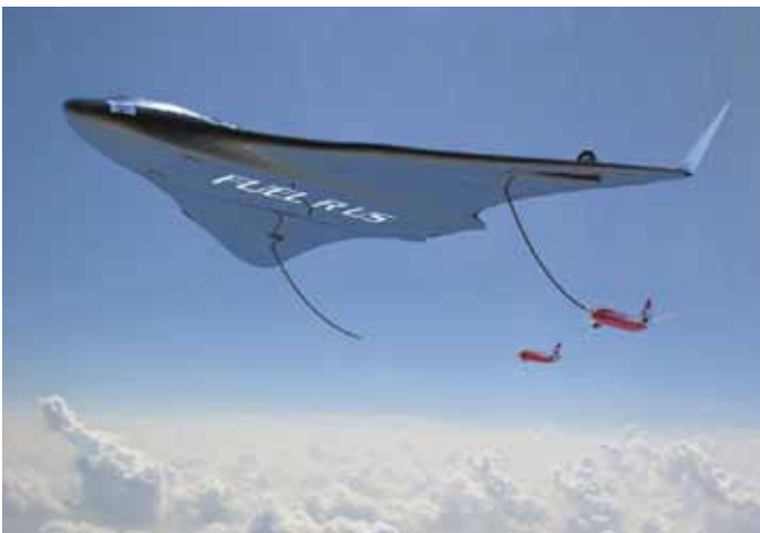
Figure 10: Artist impression of a green flight concept "air-to-air refuelling of civil aircraft" (copyright NLR)
