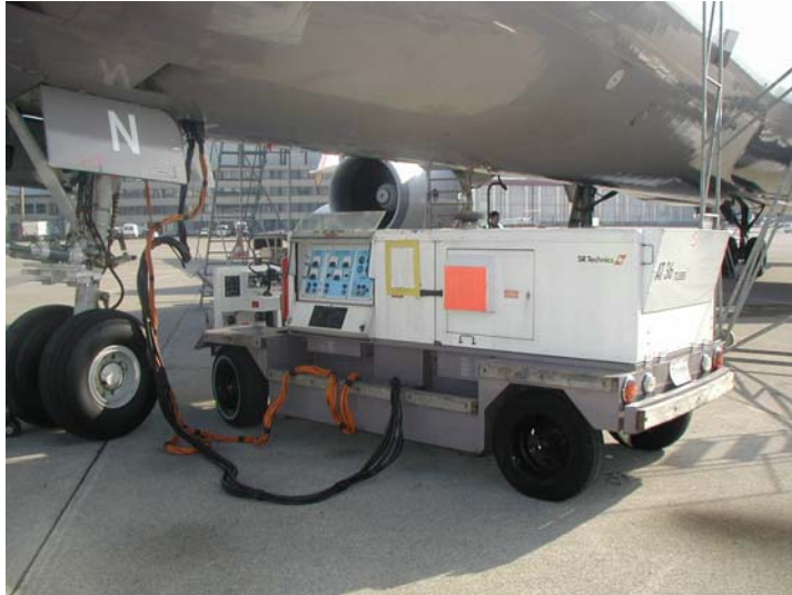
Figure 5-3: GPU for electrical power
